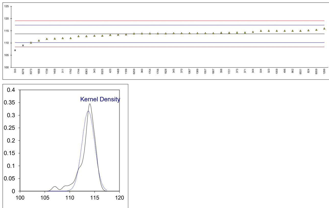
Determination of Kinematic Viscosity at 40 °C on sample #23205; results in mm<sup>2</sup>/s
